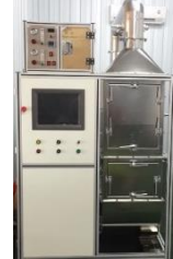
Cabin filter test
